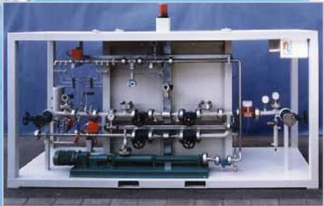
**The emulsification unit is installed on the main fuel oil line. Water, PentoMuls and PentoMag are emulsified online. The water monitor constantly monitors and regulates the water content in the emulsion.**
