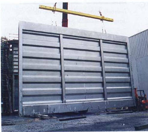
A WahlcoMetroflex Engineered Blade is lifted into the frame during shop erection. This blade is approximately 32 ft. x 20 ft. (9800 mm x 6100 mm). The two channels through the blade membrane provide both blade strength and needed seal air flow paths to the lower channel.
