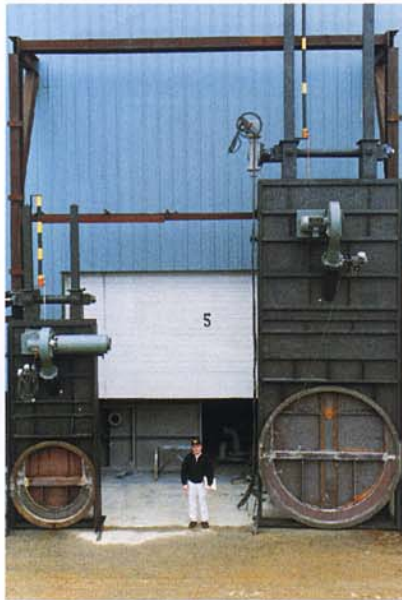
The Flex-Seal seal and blade perimeter can easily be formed for round ducts. Note the blade position indicator for verification of the blade position.
