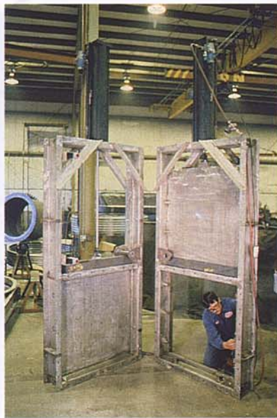
For applications where a small amount of leakage is acceptable, a slide gate is a low cost option. The design pictured above includes a locking pin to prevent inadvertent movement of the blade, and a pneumatic operator.
