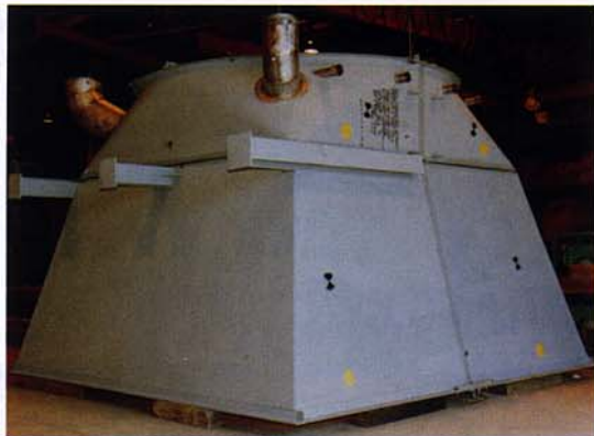
This round-to-square transition is mounted at the turbine flange. Drain connections and measurement ports are shown.
