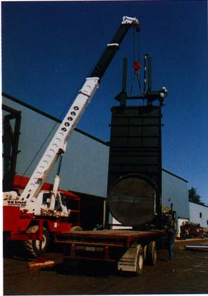
A WahlcoMetroflex guillotine is prepared for shipment. Our blade design can easily accommodate round, square or rectangular duct openings.
