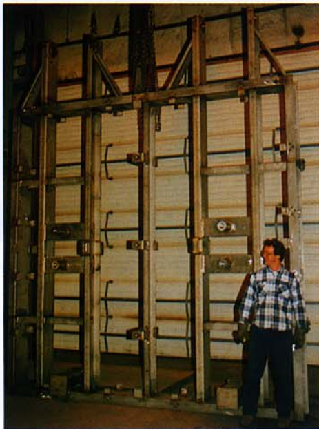
Pictured above is the blade frame for a WDV-TE-7A (toggle drive) blade.
