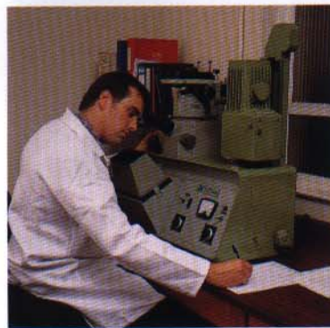
A technician using a projection microscope to verify the acceptance standards of a bellows component.
